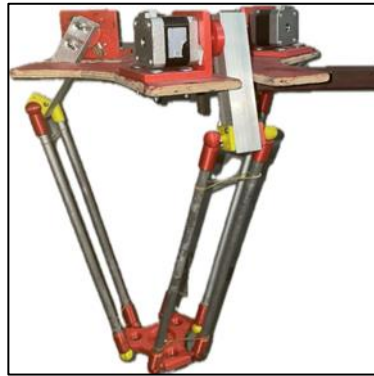
Figure 5. Delta Arm for Automated Waste Sorting
