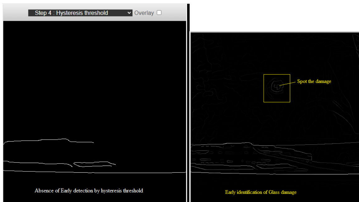
Figure 4. Two different extracted features that indicate crack in the glass
