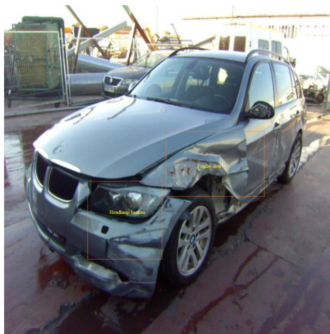
Figure 3. Detected damage area and classified results
