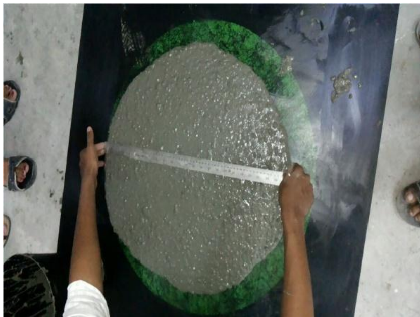
Figure 1. Flow Table Test
