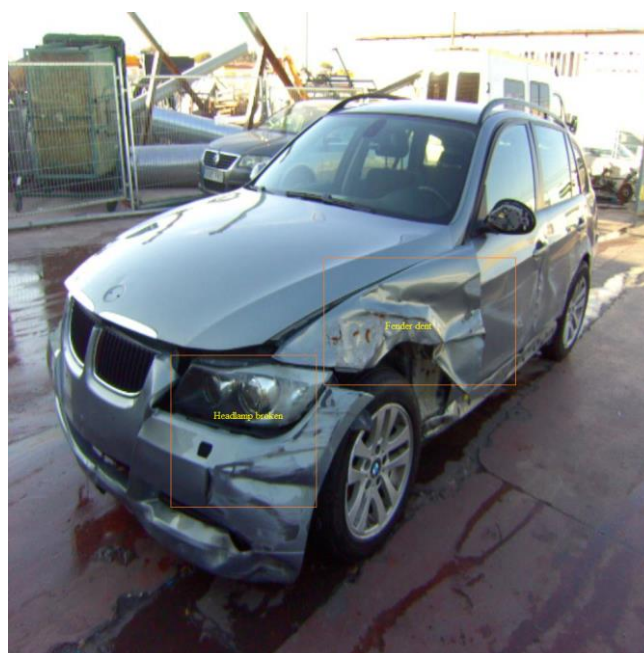
Figure 3. Detected damage area and classified results
