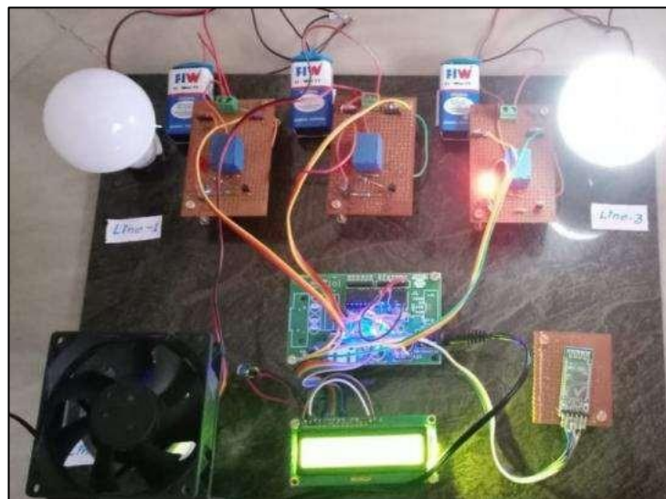
Figure 4. Experimental Setup of the Android-Based Circuit Breaker Prototype
