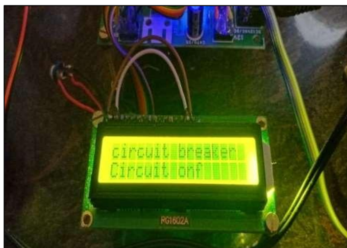
Figure 5. LCD Display Showing Real-Time Circuit Breaker Status
