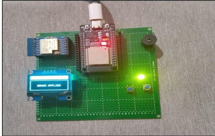
Figure 4. Experimental Setup for LoRa-Based V2V Communication Validation
