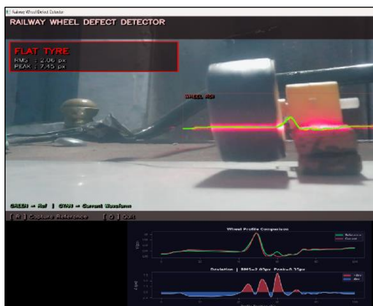
Figure 4. Image Processing Pipeline for Extracting the Wheel Profile
