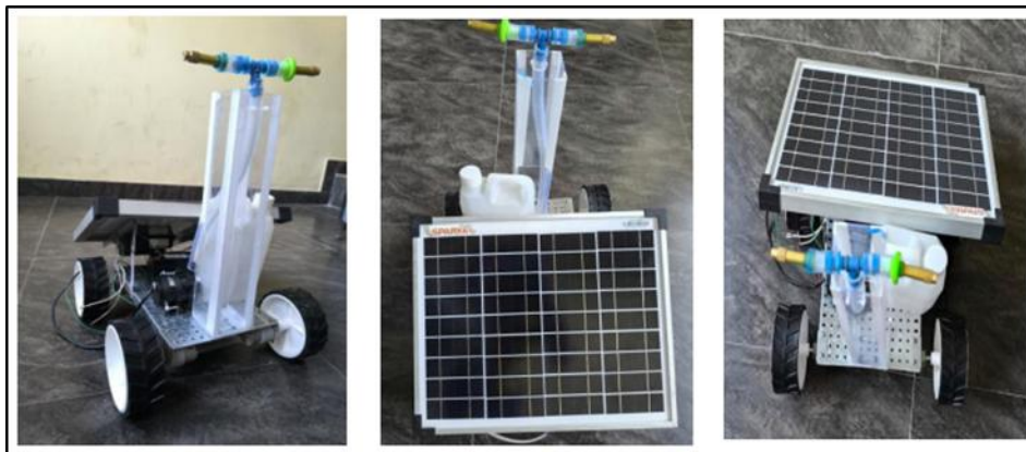
Figure 2. Fabricated IoT-based Solar-powered fertilizer sprayer prototype
