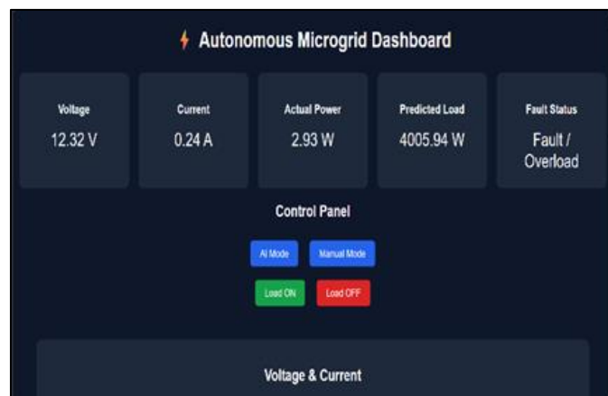
Figure 4. Real-time monitoring dashboard displaying electrical parameters and system status
