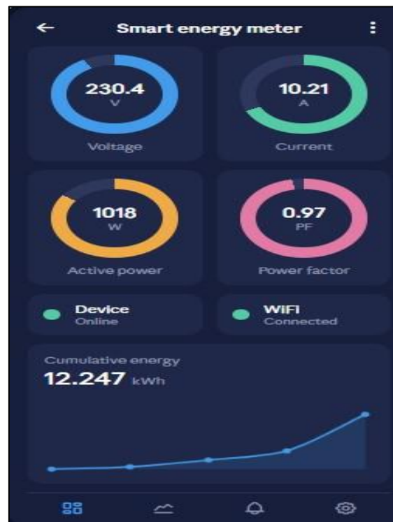
Figure 4. Blynk dashboard for real-time smart energy monitoring
