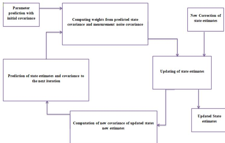
**Figure 1.** Updating state estimate with correction
