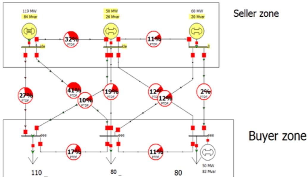
**Figure 2.** Normal load power flow in the system
