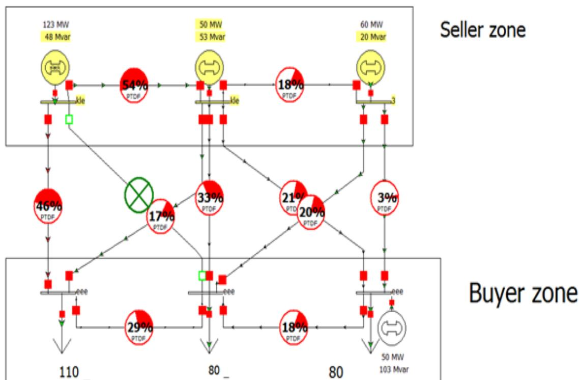
**Figure 3.** Load flow under line outage condition between bus 1 & 5
