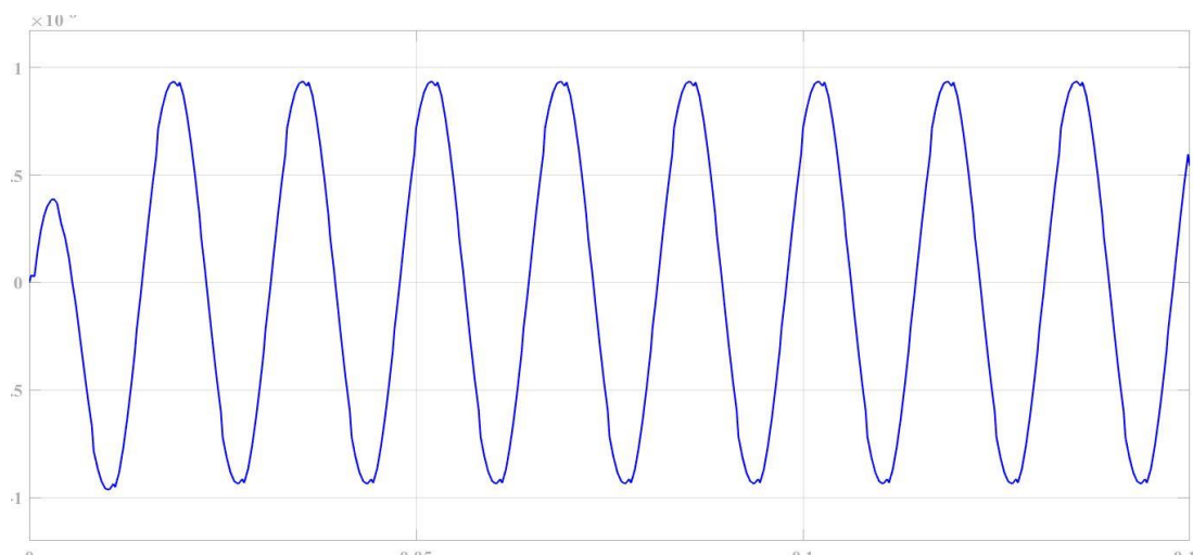
Figure 7. Leakage current flow under LG fault
