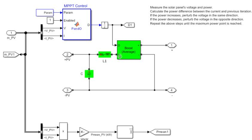
**Figure 2.** Maximum Power Point Tracking in MATLAB
