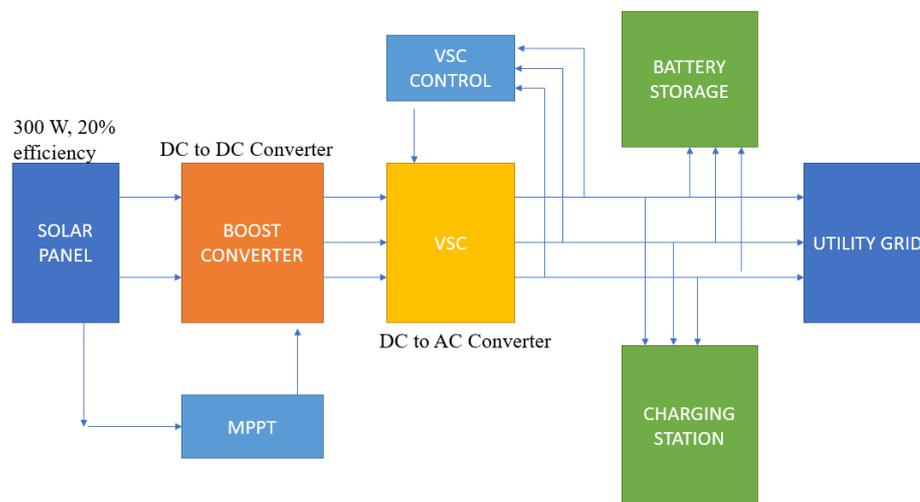
**Figure 1.** Block Diagram of Solar Powered Charging Station
