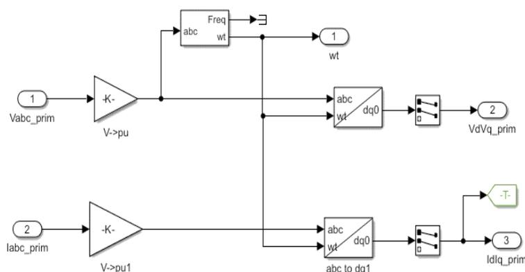
**Figure 4.** Voltage and Current Conversion
