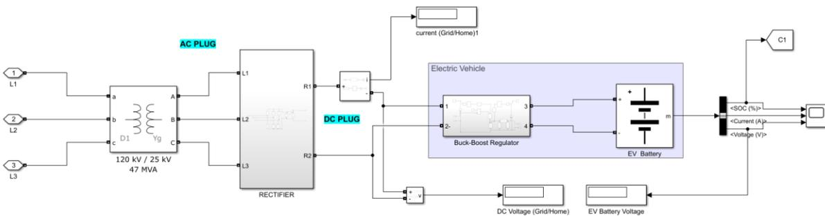
**Figure 6.** Integrated EV Charging Station
