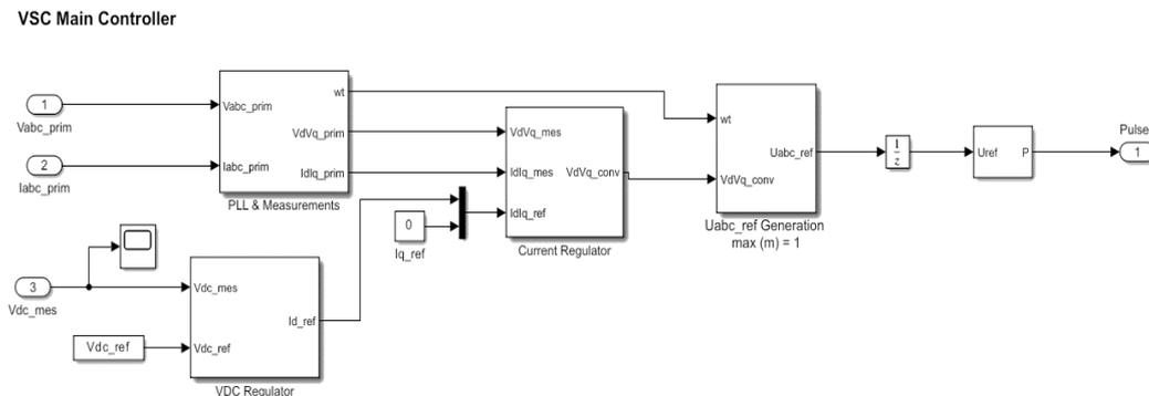
**Figure 3.** MATLAB model of VSC control
