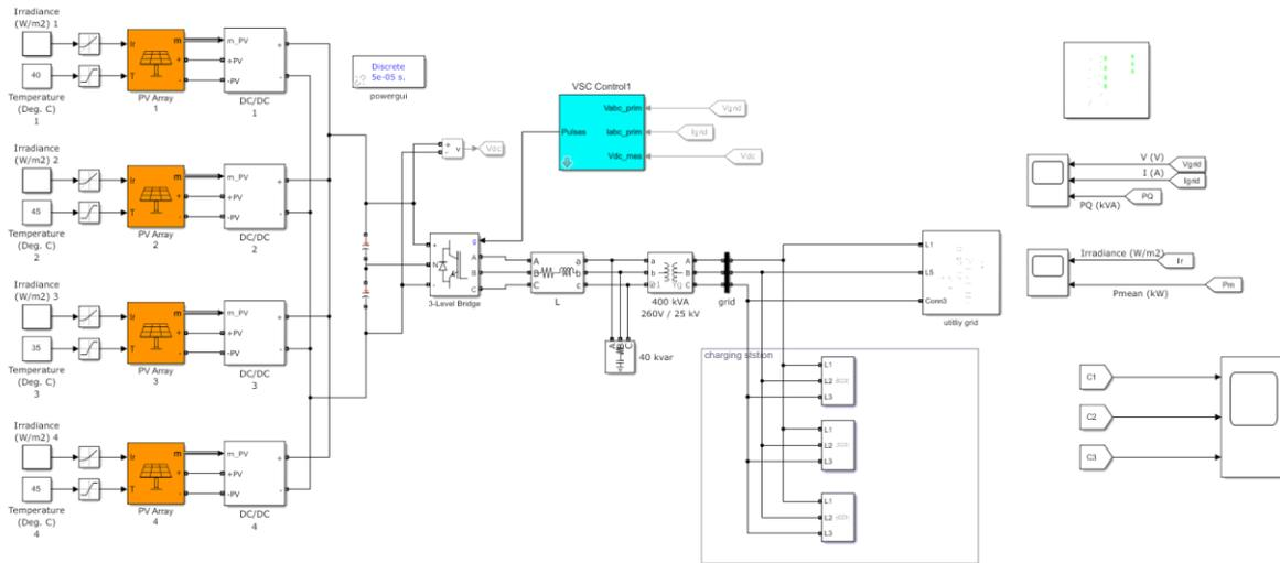
**Figure 5.** Model of 400 kW Solar Powered Charging Station for Electric Vehicle
