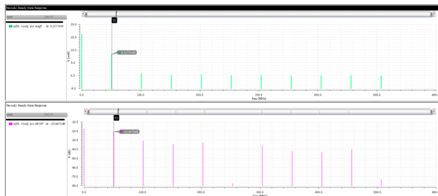
Figure 12. PSS Analysis of 5 Stage Ring Oscillator
