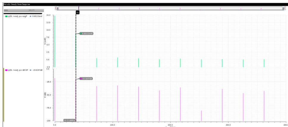
Figure 15. PSS Analysis of 7 Stage Ring Oscillator
