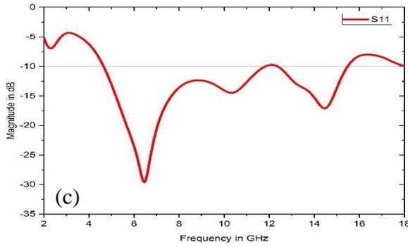
**Figure 2. (c)** Extracted  $S_{11}$  Parameter
