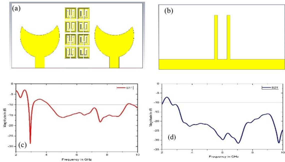
**Figure 5.** Proposed Design (a) Front View (b) Bottom View (c) Extracted  $S_{11}$  Parameter (d) Extracted  $S_{21}$  Parameter
