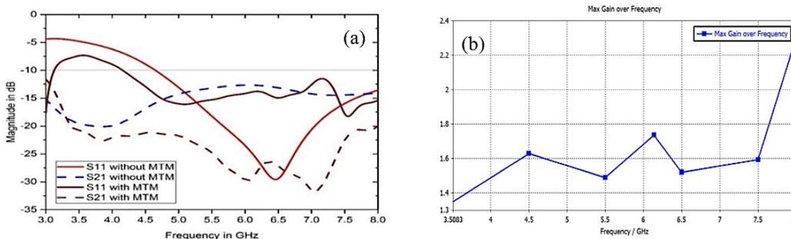
**Figure 7. (a)** Assessment S Parameter of with and without Metamaterial **(b)** Gain of the Crescent-Shaped Antenna with Metamaterial
