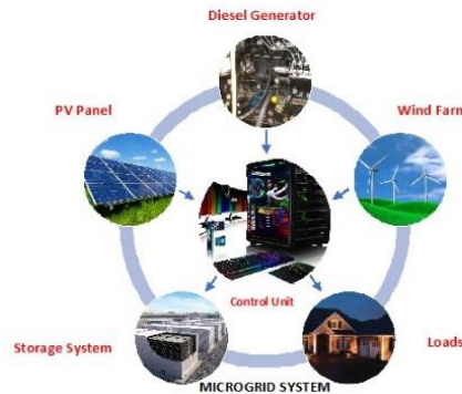
Figure 1. Illustrative Representation of MG System [16]
