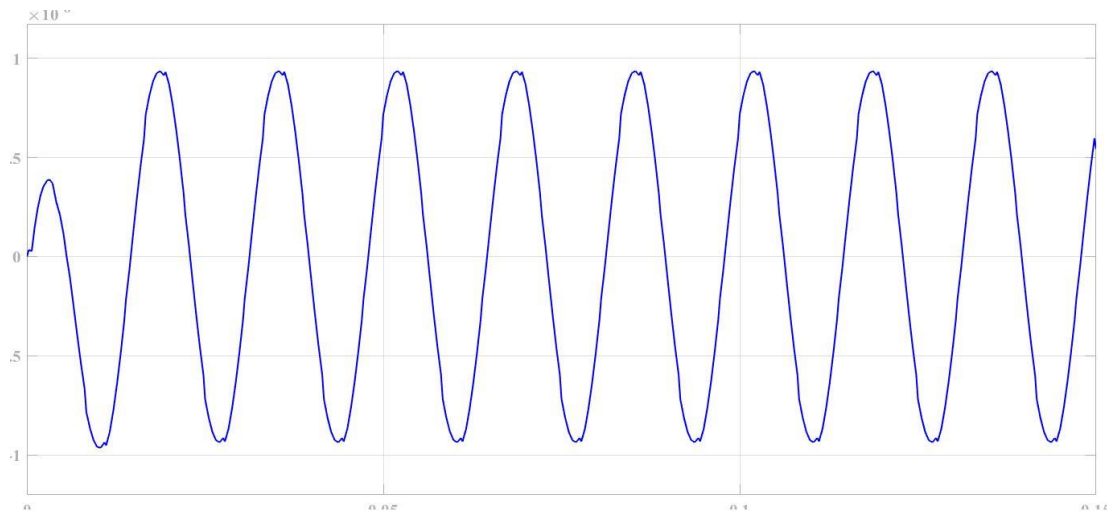
Figure 7. Leakage current flow under LG fault
