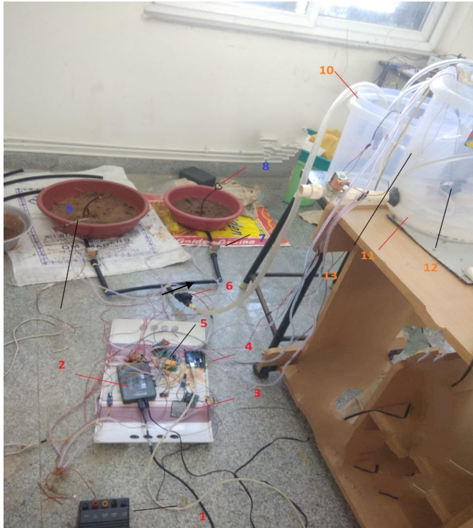
Figure 4. Prototype of the complete project (Power supply is indicated by (1) , myRIO is indicated by (2), rain sensor is indicated by (3), (4) indicates rain sensor Arduino Uno, (5) indicates 2 channel 12v relay, flow sensor is indicated by (6), (7) indicates solenoid valve, (8) indicates sprinkler, (9) indicates moisture sensor, (10) indicates bottom tank, (11) indicates top tank, (12) indicates motor, and (13) indicates level sensor.)
