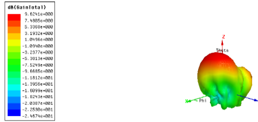
Figure 6.16. Maximum Gain at 11.1GHz
