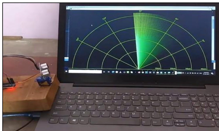
Figure 3. 360° Obstacle Detection using Ultrasonic Sensor with Servo Scanning
