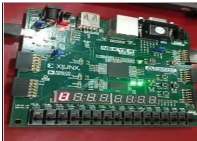
Figure 2. Nexys DDR Development Board with Xilinx Artix-7 FPGA
