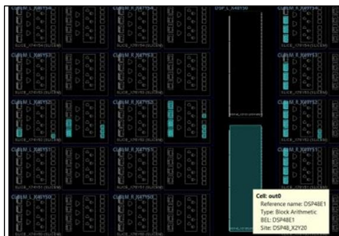
Figure 3. Place-and-Route Floorplan of the Synthesized Self-Attention Accelerator on the Artix-7
