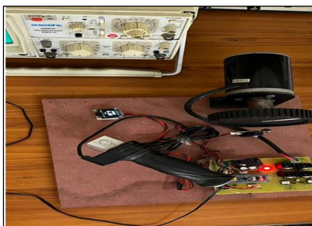
Figure 2. E-bike speed control system using STM32 microcontroller and PWM feedback
