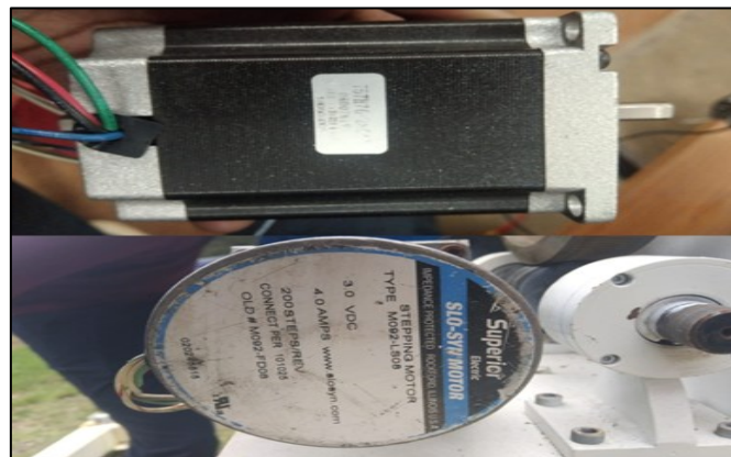
Figure 3. Stepper motor with 1:410 gear reduction assembly used in the coelostat.
