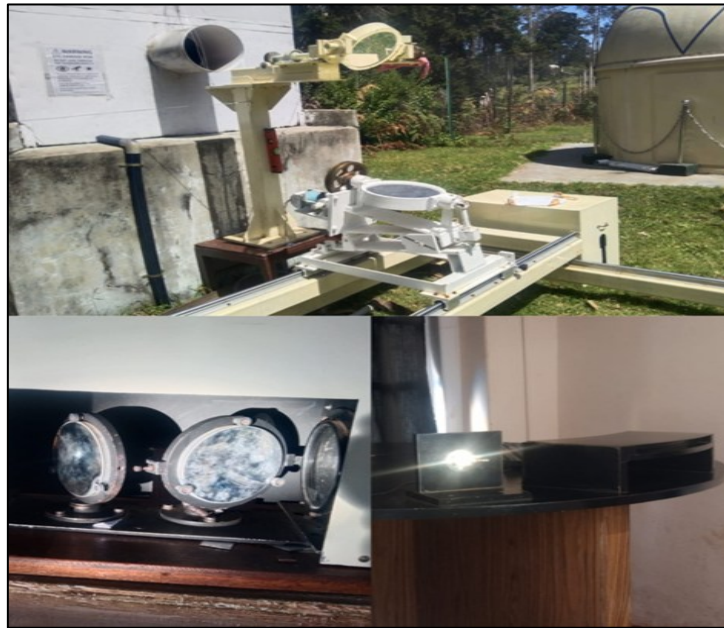
Figure 4. Installed coelostat system in museum environment.
