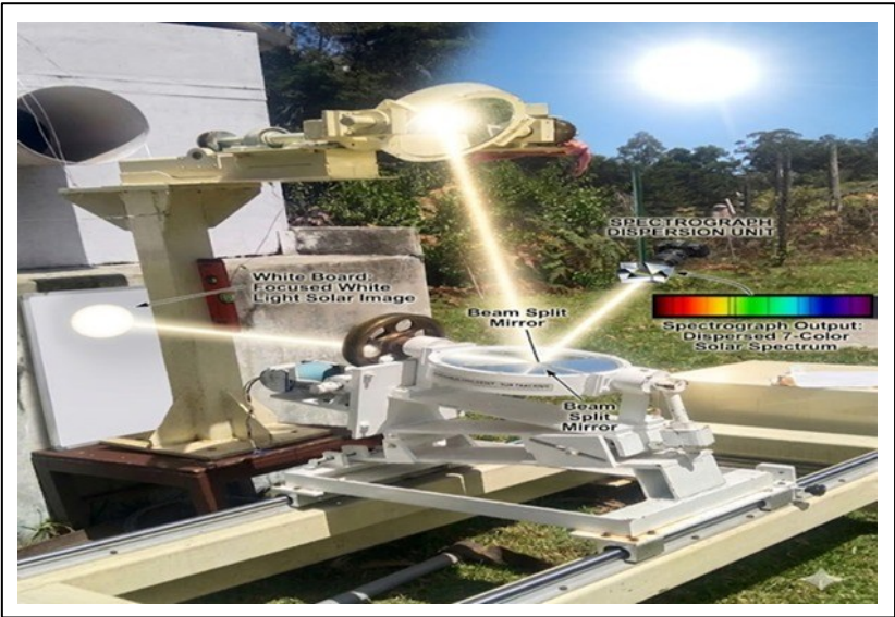
Figure 2. Optical configuration of the proposed coelostat.
