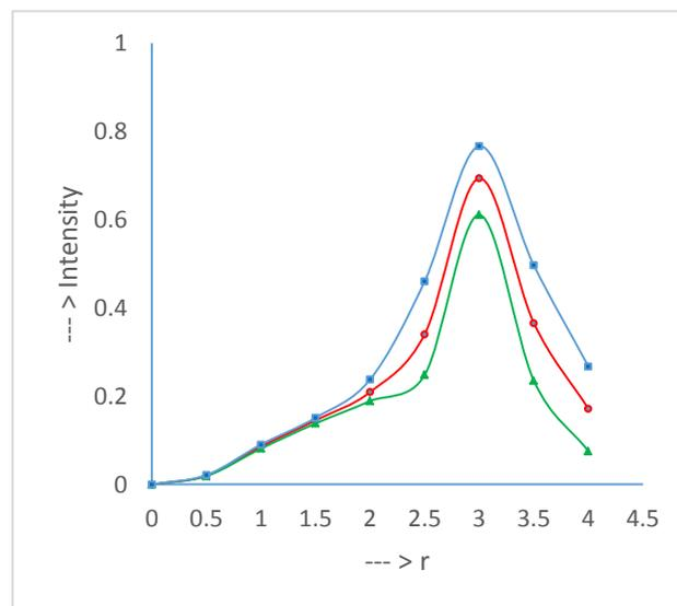
**Fig.4.** Distribution of intensity'  $\Psi^2(r)$  for signal at wavelength of 1550 nm for  $LP_{11}$  mode in an EDFA consisting of Trapezoidal-index fiber with  $S= 0.5, V = 3.1, a = 3\mu\text{m}, NA = 0.2548$  for different nonlinearity parameters  $n_{NL}P$  (Our results:  $\blacktriangle$  for  $n_{NL}P = +1.5 \times 10^{-14} \text{m}^2$ ,  $\bullet$  for  $n_{NL}P = 0$  and  $\blacksquare$  for  $n_{NL}P = -1.5 \times 10^{-14} \text{m}^2$ ; — simulated exact results)
