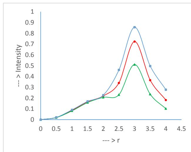
**Fig.2.** Distribution of intensity  $\Psi^2(r)$  for pump at wavelength of 1480 nm for  $LP_{11}$  mode in an EDFA consisting of Trapezoidal-index fiber with “ $S= 0.5, V = 3.25, a = 3\mu m, NA = 0.2550$  for different nonlinearity parameters  $n_{NL}P$  (Our results:  $\blacktriangle$  for  $n_{NL}P = +1.5 \times 10^{-14} m^2$ ,  $\bullet$  for  $n_{NL}P = 0$  and  $\blacksquare$  for  $n_{NL}P = -1.5 \times 10^{-14} m^2$ ; — simulated exact results)”
