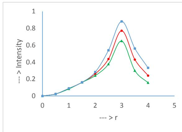
**Fig.3.** Distribution of intensity'  $\Psi^2(r)$  for signal at wavelength of 1550 nm for  $LP_{11}$  mode in an EDFA consisting of Trapezoidal-index fiber with  $S= 0.25, V = 3.8183, a = 3\mu\text{m}, NA = 0.3138$  for different nonlinearity parameters  $n_{NL}P$  (Our results:  $\blacktriangle$  for  $n_{NL}P = +1.5 \times 10^{-14} \text{m}^2$ ,  $\bullet$  for  $n_{NL}P = 0$  and  $\blacksquare$  for  $n_{NL}P = -1.5 \times 10^{-14} \text{m}^2$ ; — simulated exact results)
