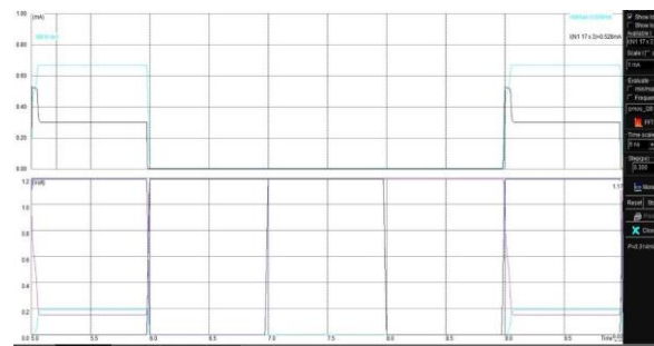
Figure 16. Power Analysis of 6T SRAM (32nm) During WRITE
