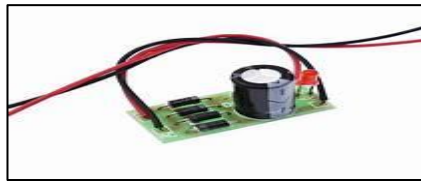
Figure 5. AC to DC Converter
