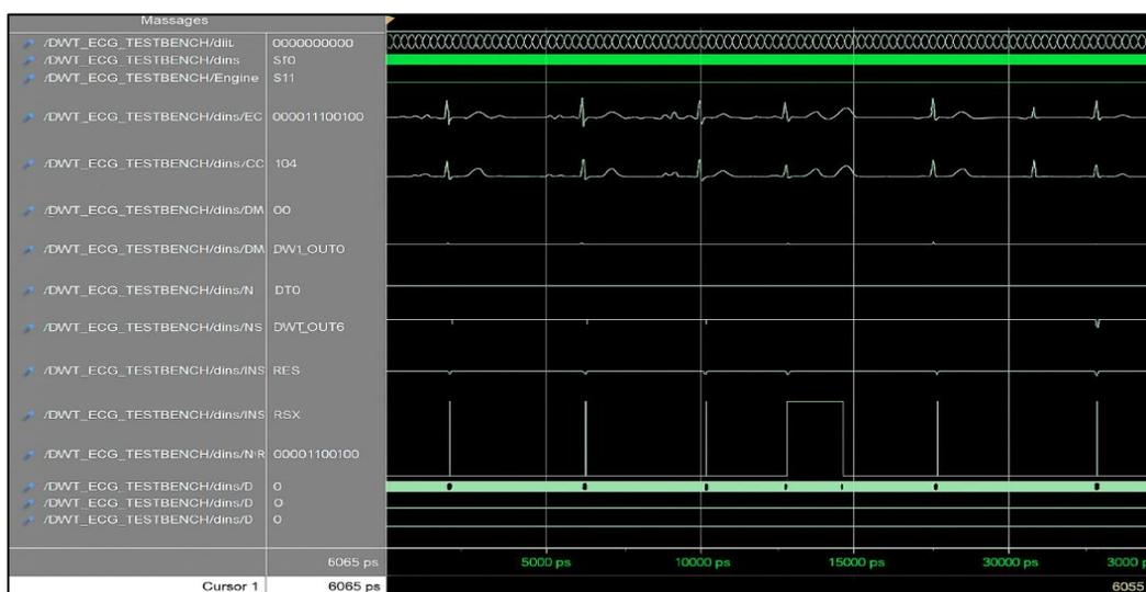
**Figure 6(a).** ModelSim Simulation Waveform of the Proposed Lifting-based DWT Architecture for ECG Denoising
