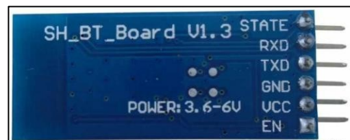
Figure 6. Bluetooth module HC-05 Figure 7. Bluetooth Module HC-05 Pin Diagram
