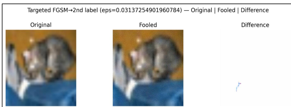
Figure 4. Targeted FGSM (target = second-most-likely clean label) at \epsilon = 8/255 : Original image, adversarial image, and contrast-enhanced perturbation map.
