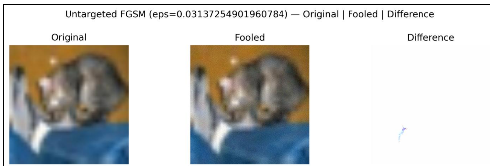
Figure 3. Untargeted FGSM examples at \epsilon = 8/255 : Original image, adversarial image, and contrast-enhanced perturbation map.
