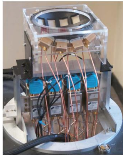
Figure 2. Setup of Ultra-Wideband Radar for Detection of Breast Cancer [5].
