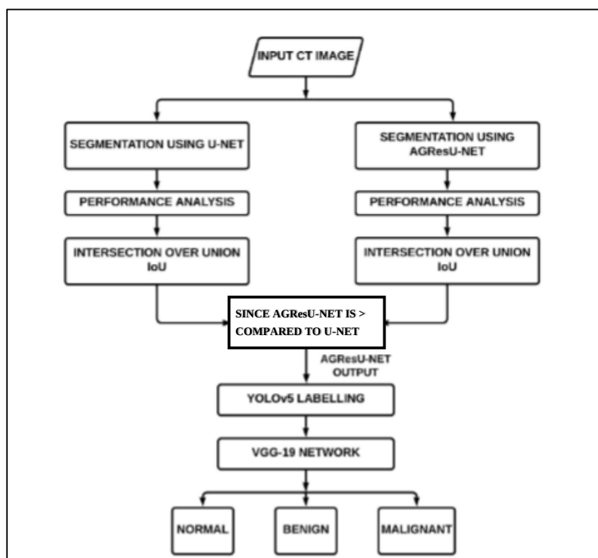
Figure 3. Process Diagram for Segmentation and Identification of Lung Tumor
