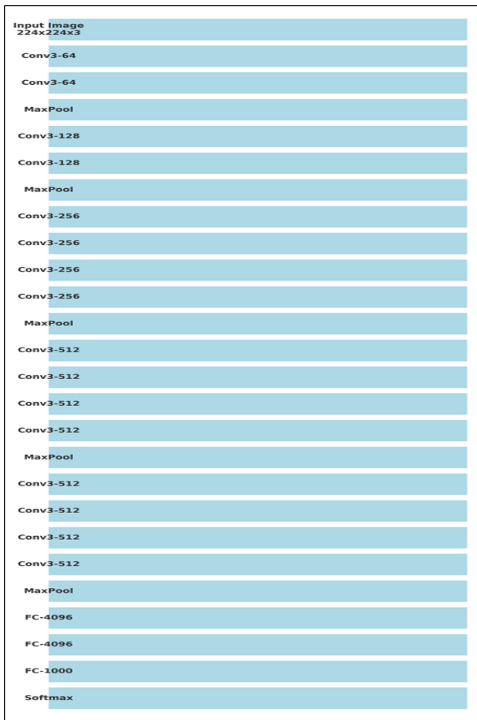
Figure 7. Visualizing VGG-19: Layers, Convolutions, and Max-Pooling
