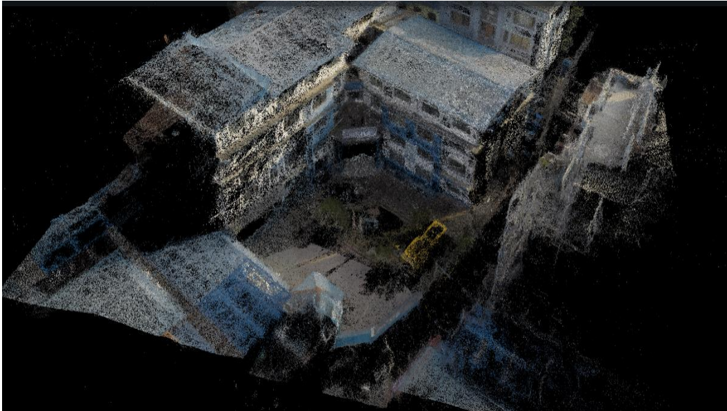
Figure 12. Point Cloud Estimation of Data from the Images
