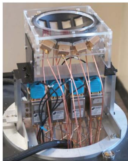
Figure 2. Setup of Ultra-Wideband Radar for Detection of Breast Cancer [5].
