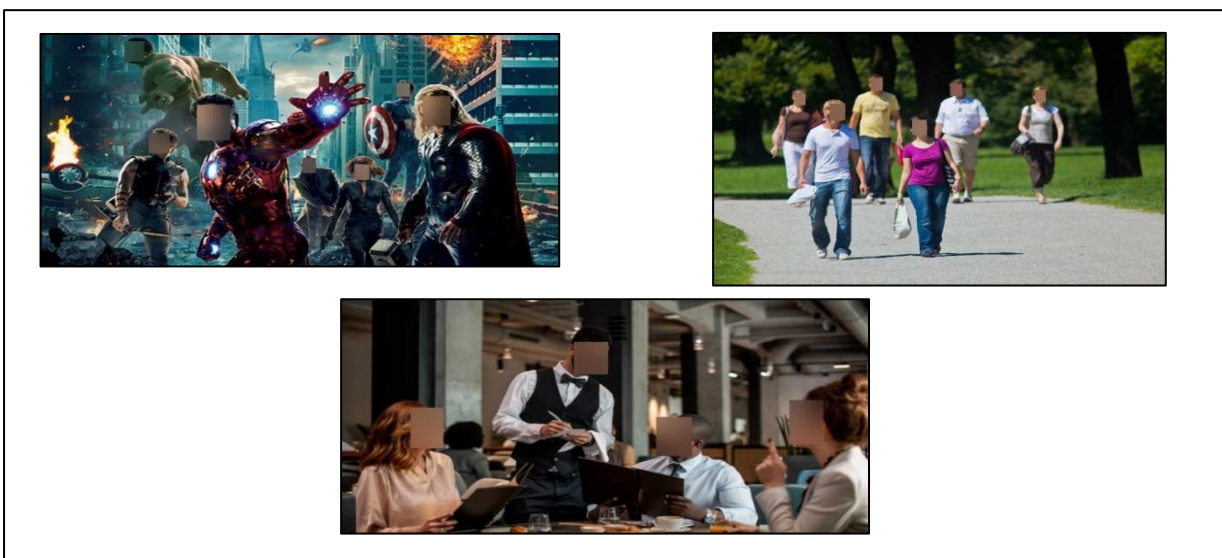
Figure 6. Faces Detected and Blurred from the Image.
