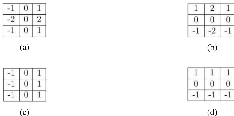
Figure 5: (a) and (b) display the Sobel kernels (Vertical and Horizontal), respectively, while (c) and (d) show the Prewitt kernels (Vertical and Horizontal), respectively.
