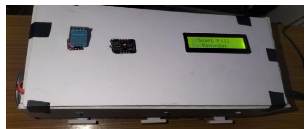
Figure 14. Top View Showing MAX30102 and DHT11 Sensors
