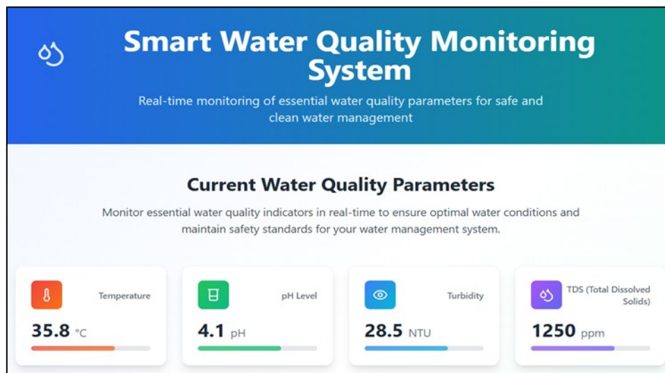
Figure 9. Dashboard Showing Real-Time Water Quality Data
