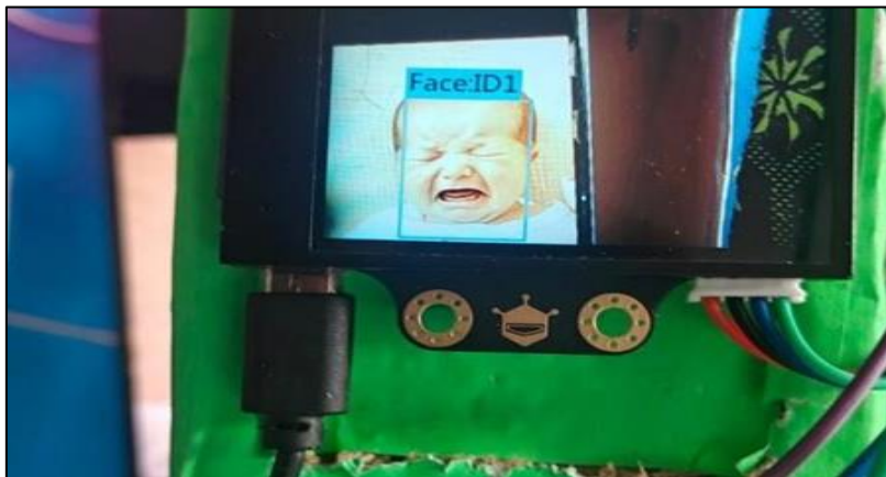
Figure 3. Infant Cry Detection Using HuskyLens AI Vision Sensor
