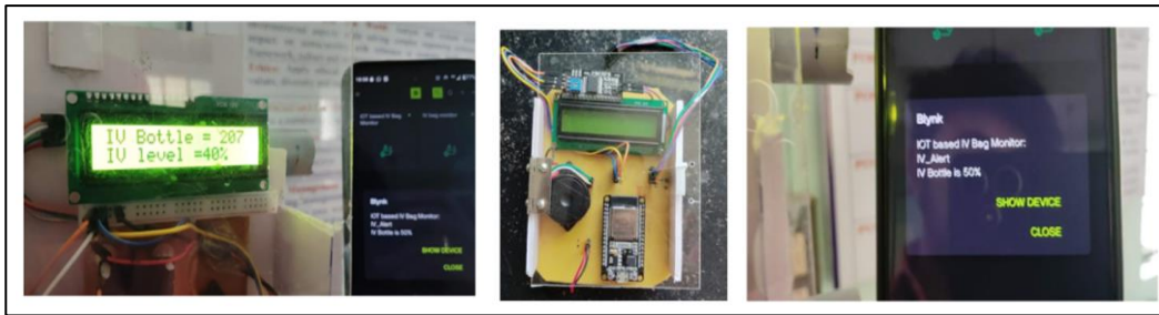
Figure 5. Real-Time Monitoring and Alert Validation of the Proposed IV Fluid Monitoring System
