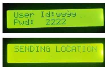
Figure 5. Password Verification Process
