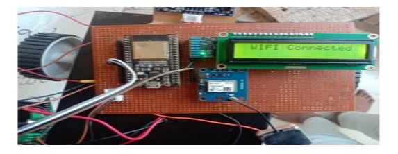
Figure 4.1. The Car Unit Connected to the Internet
