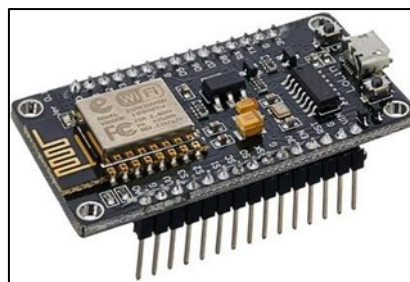
Figure 4. AI Integrated Microcontroller ESP8266 NodeMCU Board
