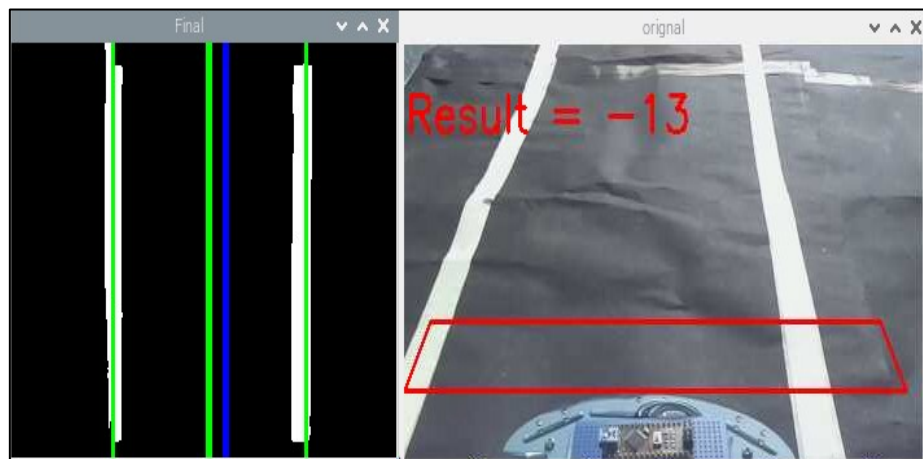
Figure 4: Output Showing the Offset When Car is Slightly Right
