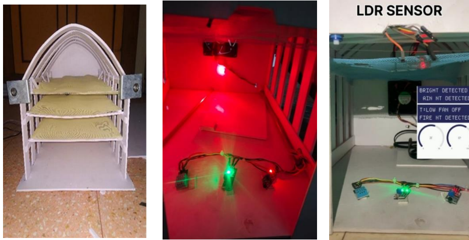
Figure 4.3, Hardware model of the dehydration shed control system
