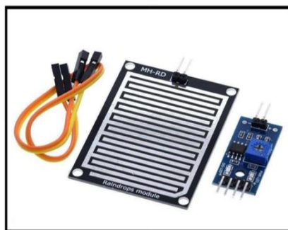
Figure 3.2.4. Rain Fall Sensor
