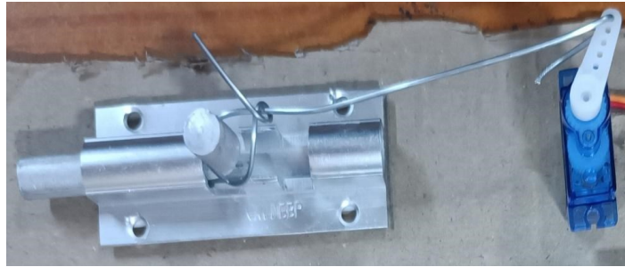
Figure 10. Interfacing Lock with Servo
