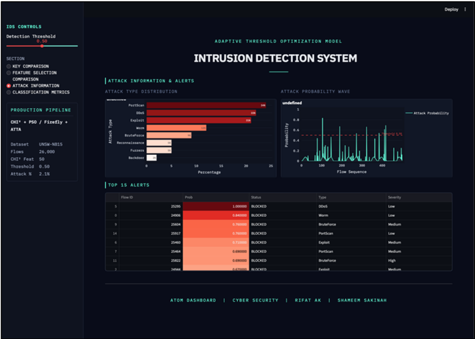
Figure 8. Attack detection dashboard showing attack distribution, alert table, and probability analysis
