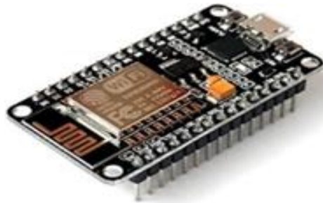
Figure 3. Node MCU Microcontroller Plus Wi-Fi
